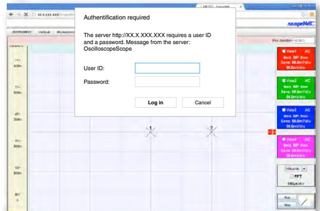
3 Two methods can be used to manage all the oscilloscopes: clicking directly on the menu bar to change the parameter settings of all the instruments in one go or clicking directly on the name of the instrument which you want to configure.
